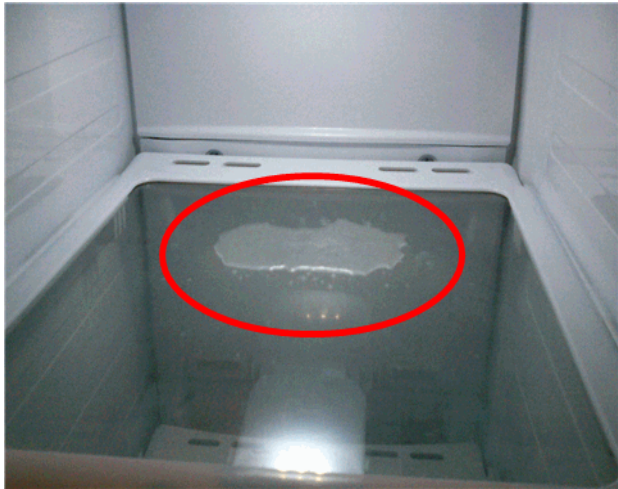
The refrigerator's ice maker appeared to be leaking.
